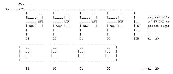
SW indicates a switch, where the up position corresponds to HI and the down position to LO. The O encased in a rectangle connected to the strobe input is the button used to strobe from low to high to allow the display to accept the current inputs. To set the second-left digit to 6, for example, the switches must be in positions [down up up down] and A1 must be connected to power while A0 remains connected to ground. Then press the strobe button and the digit will appear.
